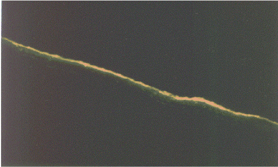
Figure 3.23: Fluorescence of the bleached ICG layer (6.45 mM) after irradiation with one pulse of 55 \text{ mJ/mm}^2 . Thickness of the fluorescing layer was 10 \mu\text{m} .
