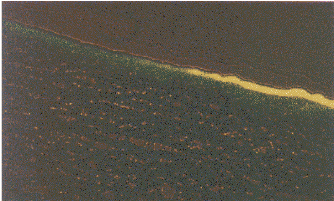
Figure 3.22: The picture shows the contrast between unirradiated control portion on the left and bleached portion on the right. The sample was stained with 6.45 mM ICG solution. The bright fluorescing portion was irradiated with 5 pulses of 55\ \text{mJ}/\text{mm}^2 .
