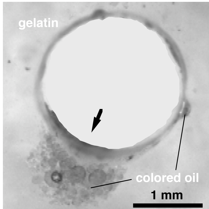
Figure 6.4: Top view of colored-oil distribution in a 2 mm channel through gelatin (175 bloom) with cylindrical geometry after 50 pulses of 40 mJ laser energy through a side-firing fiber in 300\text{ cm}^{-1} colored oil. The laser energy was delivered perpendicular to the channel wall as indicated by the arrow.
